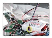
11. Connect GPS cable to GPS port of FCS-H500 main controller again.
