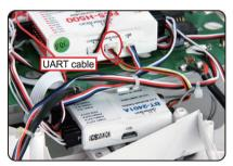
Connect UART cable to the DATA PORT of FCS-H500 main controller, and fix the BT-2401A (BT-2402A) ready.
