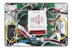
The installation instruction map of RX705(RX708) receiver and BT-2401A(BT-2402A).
