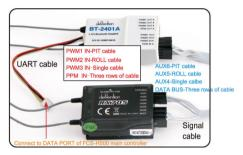
5. Using signal cable to connect BT-2401A(BT-2402A) with RX705(RX708) receiver.
