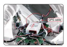
Take down the upper cover of TALI H500 and the connect wire which connected FCS-H500 main controller with GPS port.
