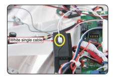
Reconnect the white single cable with TELEMETRY CON on the RX705(RX708) and fix the receiver.
