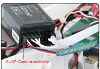
Reconnect the camera controller with AUX7 on the RX705(RX708).
