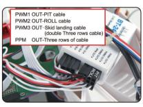
Connect the gimbal cable (used to connect receiver), DATA BUS cable and cable for skid landing to BT-2401A(BT-2402A).
